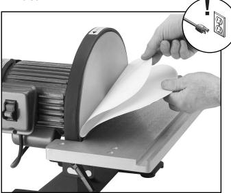
**Figure 6**. Removing protective layer.
